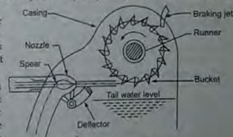
Fig. 6.5. Elements of a Pelton wheel
